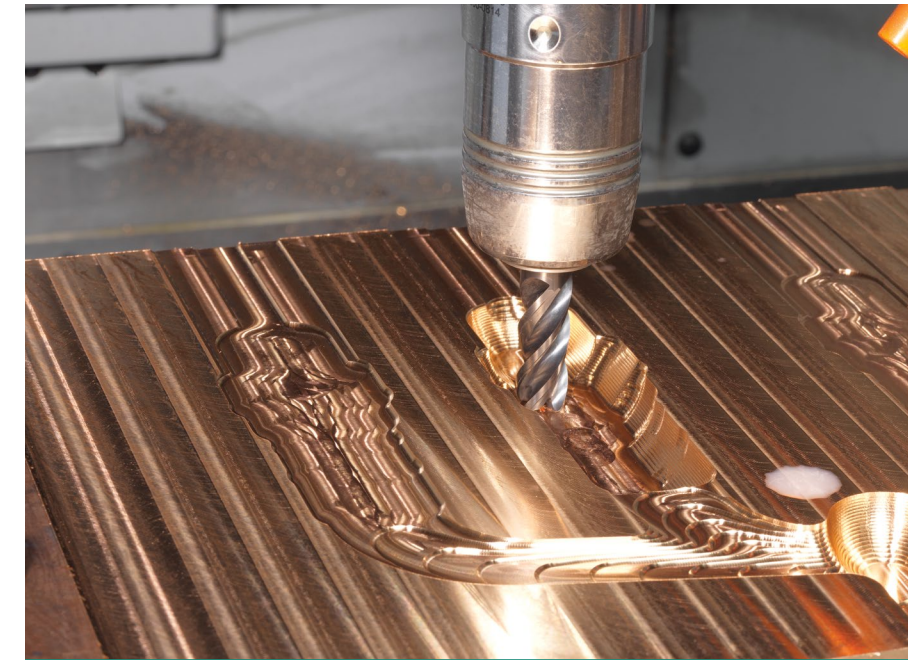
The enhanced spindle power and expanded work zone of the PS95 has enabled Chicago Faucets to reduce cycle times by 50 percent, taking and producing both mating cavities of a tool in one setup.
